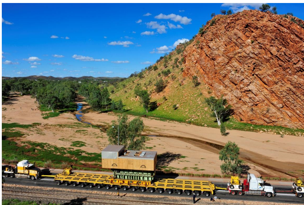
The 51/60DF dual-fuel engine pictured on its low-loader on the journey between Darwin and Owen Springs, Australia
