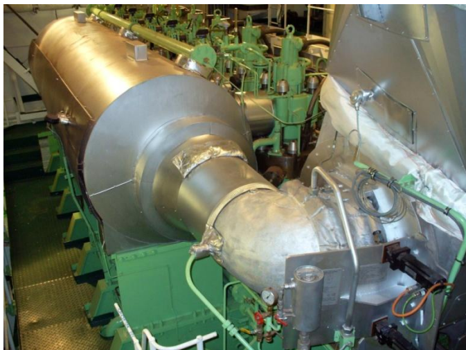
The MAN Diesel VTA system aboard the shallow draught tanker Stena President. The field test followed extensive test-bed testing on the six cylinder, 46 cm bore 6S46MC-C engine at MAN Diesel's Croatian licensee Brodosplit.
