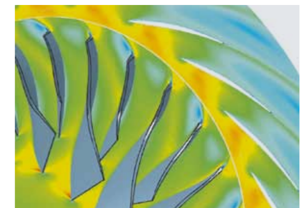
Pressure and mach number distribution
